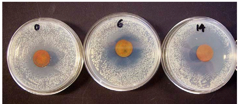
Figure 3 Inhibition of bacteria due to the presence of copper coins. The coins were placed on the bacterial growth media (Nutrient Agar) at various times (0, 6, and 14 hours) before the bacteria were applied.
