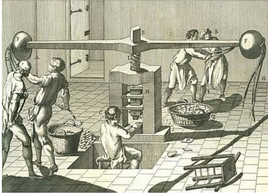
Figure 2.17 – Diderot and d’Alembert. Monnoyage – Balancier . 1772. Depiction of a screw press in use to make coins.
