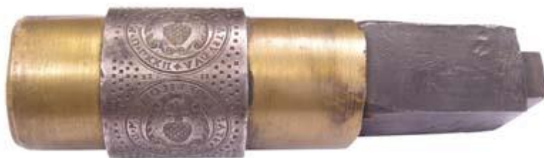
Figure 2.15 – A roller die from the Augsburg mint in Germany (www.segoviamint.org)
